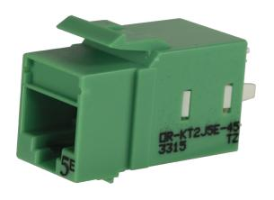
Category 5e Keystone jack, 8-position, 180 degree exit, icon compatible, T568A/B wiring, Green , individually packaged. Keystone, KT2J jacks and modules feature New installer friendly lacing cap termination with free termination tool in every carton. The keystone footprint allows flexibility in installation scheduling because its rear insertion into the faceplate allows the technician to complete the termination before and during the construction process.
