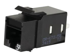
KT2J jacks, available in CAT6A, CAT6 and CAT5E, represent the next generation of keystone termination. These jacks utilize an installer friendly lacing cap termination. Termination tool supplied with every carton of 20 or bulk pack of 25.
