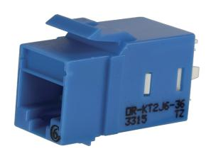
Category 6 Keystone jack, 8-position, 180 degree exit, icon compatible, T568A/B wiring, Blue, individually packaged. Keystone, KT2Jjacks and modules feature New installer friendly lacing cap termination with free termination tool in every carton. The keystone footprint allows flexibility in installation scheduling because its rear insertion into the faceplate allows the technician to complete the termination before and during the construction process.
