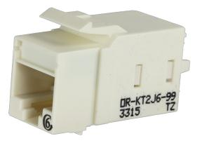
Category 6 Keystone jack, 8-position, 180 degree exit, icon compatible, T568A/B wiring, White , individually packaged.Keystone, KT2J jacks and modules feature New installer friendly lacing cap termination with free termination tool in every carton. The keystone footprint allows flexibility in installation scheduling because its rear insertion into the faceplate allows the technician to complete the termination before and during the construction process.
