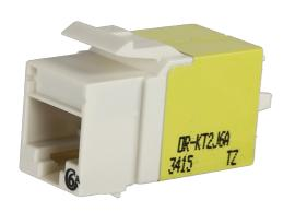
Category 6A Keystone jack, 8-position, 180 degree exit, icon compatible, T568A/B wiring, Fog White, individually packaged. Keystone, KT2J jacks and modules feature New installer friendly lacing cap termination with free termination tool in every carton. The keystone footprint allows flexibility in installation scheduling because its rear insertion into the faceplate allows the technician to complete the termination before and during the construction process.
