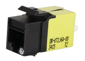
Category 6A Keystone jack, 8-position, 180 degree exit, icon compatible, T568A/B wiring, Black, individually packaged. Keystone, KT2J jacks and modules feature New installer friendly lacing cap termination with free termination tool in every carton. The keystone footprint allows flexibility in installation scheduling because its rear insertion into the faceplate allows the technician to complete the termination before and during the construction process.
