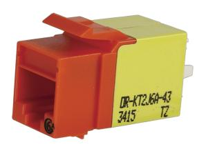
Category 6A Keystone jack, 8-position, 180 degree exit, icon compatible, T568A/B wiring, Orange, individually packaged. Keystone, KT2J jacks and modules feature New installer friendly lacing cap termination with free termination tool in every carton. The keystone footprint allows flexibility in installation scheduling because its rear insertion into the faceplate allows the technician to complete the termination before and during the construction process.
