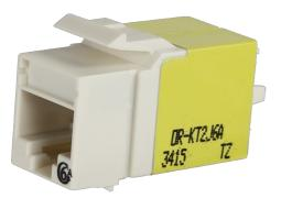
Resealable package of 25 Category 6A Keystone jack, 8-position, 180 degree exit, icon compatible, T568A/B wiring, Fog White. Keystone, KT2J jacks and modules feature New installer friendly lacing cap termination with free termination tool in every carton. The keystone footprint allows flexibility in installation scheduling because its rear insertion into the faceplate allows the technician to complete the termination before and during the construction process.
