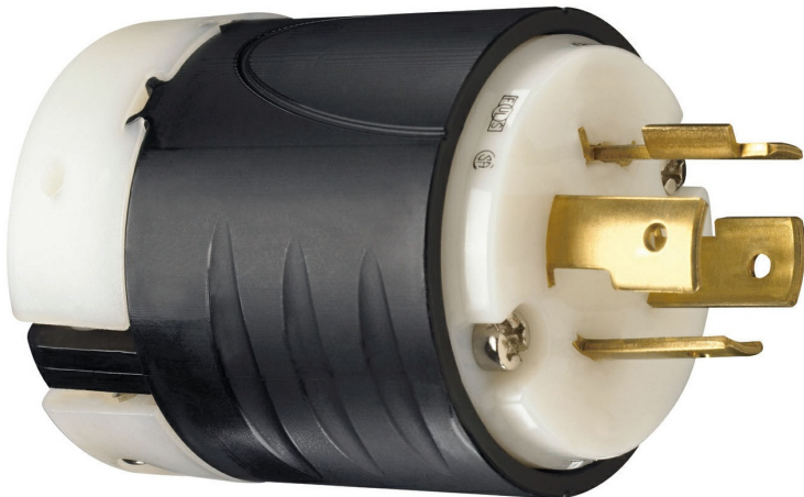
Turnlok® Plug 4-Wire 20A 125/250V
