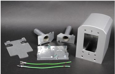
Aluminum housing and side plates, with a steel base and divider, measures 4" x 5" x 5 5/8". Base is configurable to have a combination of two 3/4" knockouts or two 3/4" EMT stubs. Accommodates a variety of power outlets (duplex, decorator, GFCI and up to 30A twist lock). Use Wiremold AVIP to provide communications and A/V. Receptacles and wall plates are sold separately.
