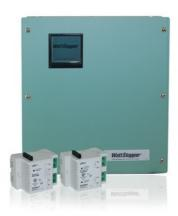
The LCDP-1 is a relay module designed for use and easy installation within the LC8-120/277 panel. The LCDP-1 is a double pole/single relay module with one 20 amp relay and voltage of 208, 240, or 480 VAC.
