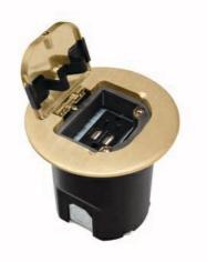
A round wood floor box kit with a brass finish that supplies power in open space living. The receptacle includes USB Type A charging that will supply 3.1A to power all mobile devices. It can be installed on carpet, wood, natural stone and tile floors that have a wooden subfloor.
