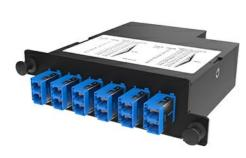
High density modular fiber optic pre-terminated cassettes provide plug-and-play functionality with the high density footprint accommodating up to 96-fibers in one rack unit.
