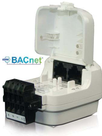
The LMBC-300 Digital Network Bridge provides a segment network connection for a group of Digital Lighting Management (DLM) local network devices. This enables individual DLM local networks to be aggregated into a larger system, which, in turn, can be remotely managed from a DLM Segment Manager or a building automation system (BAS).
