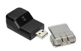
The LMCI-100 Computer to DLM interface connects to a PC's USB port running the LMCS-100 Digital Lighting Management computer software and to a Digital Lighting Management (DLM) system through the RJ45 connector. The computer tools allow users to read, store and modify DLM system configurations.
