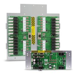
The LMCP retrofit kits provide a simple upgrade option to existing Wattstopper Lighting Integrator and other legacy relay panels (GE and Horton Controls SWC, SWS, SWSP and TLC panels). The kit is compatible with several common lighting relays, including HDR, RR7, and RR9. With the intelligence cards, the panel is fully compatible with the DLM technology platform and enables an optional MS/TP network.
