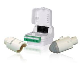
The LMIO-301 photocell input module is an accessory for a networked Digital Lighting Management (DLM) installation that allows an LMSM segment manager or LMCP panel to read ambient light levels for use in controlling exterior lighting or interior lighting installed in brightly daylit spaces such as atriums. The LMIO-301 works in conjunction with either the LMPO-200 exterior or LMPS-6000 skylight low voltage photocell heads.
