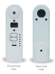
The LMLS-600 is a dual loop photosensor that automatically switches or dims one zone of lighting based on ambient light and daylight levels. It has two silicon photodiodes with an extended range of 1–10,000 footcandles (fc) and features photopic correction to mimic the human eye's perception of daylight. The LMLS-600 is part of a Digital Lighting Management (DLM) system and sends light level signals to control loads connected to DLM on/off or dimming room controllers.
