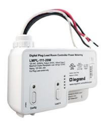
The LMPL-111-20M Plug Load Controller contains a 20 amp relay for on/ off control of connected outlets, and a highefficiency intelligent switching power supply. This plug load controller works as part of the Wattstopper Digital Lighting Management (DLM) system and enables energy-efficient control of plug loads.
