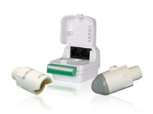
The LMIO-301 photocell input module is an accessory for a networked Digital Lighting Management (DLM) installation that allows an LMSM segment manager or LMCP panel to read ambient light levels for use in controlling exterior lighting or interior lighting installed in brightly daylit spaces such as atriums. The LMIO-301 works in conjunction with either the LMPO-200 exterior or LMPS-6000 skylight low voltage photocell heads.
