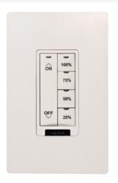
LMPW-100 Series Digital PIR Wall Switch Occupancy Sensors use passive infrared (PIR) technology to detect occupancy for energy-efficient control of lighting and plug loads. They also include one or two switch buttons for manual control of selected loads, and are part of a Wattstopper Digital Lighting Management (DLM) system
