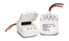
LMRC-100 Series Digital Room Controllers include one or two relay(s) for on/off control of a total of 20 amps, and a highefficiency switching power supply. They are the foundation of a Wattstopper Digital Lighting Management (DLM) system, and allow integration of occupancy sensors, daylighting sensors and switches for energyefficient lighting control.
