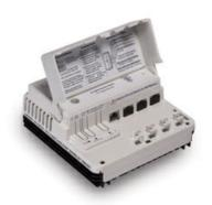
LMRC-220 Series Digital Room Controllers include one or two output(s) to control a total of up to 20 amps for certain load types. Load ratings include incandescent, magnetic low voltage, forward phase compatible electronic low voltage and LED drivers, neon and cold cathode, and dimmable two-wire and three-wire fluorescent ballasts, and E-ballasts.
