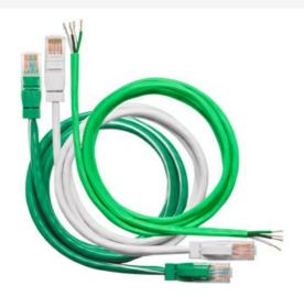
LMRJ Series cables connect Digital Lighting Management (DLM) components without the need for tools or point-to-point discrete wiring. Cables are pre-terminated with industry standard RJ45 connectors compatible with any RJ45 port on DLM components. LMRJ cables utilize B to B wiring.
