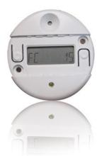
The LS-102 Daylighting Controller is a single zone, on/off switching device designed to be installed in a closed loop application. A self-contained 24 VDC device with an extended range of 1-1400 footcandles, the LS-102 requires a low voltage power pack to operate. The controller consists of an advanced digital multi-band photosensor, an on-board microcontroller, and an LCD display. This photosensor is positioned behind a 100° cone that cuts off unwanted light, preventing false triggers.
