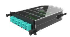
Infinium M4 Splice Cassettes enable industry leading performance, fast field termination, and provide cable management within the housing. The Splice Cassettes are designed for use with Single-Mode (OS2) or Multimode (OM4/OM5) Fiber, Houses 12-24 fibers and are available in LC Duplex or LC Quad port configurations. Compatible with Infinium HD-E Rack Mount Fiber Enclosure with M4 Drawer Face.
