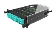
Q-Series Splice Cassettes are available in the M2 footprint. These cassettes have been engineered with innovated features to simplify install, speed-up field termination, provide cable management within the housing and ensure high performance. The Splice Cassettes are designed for use with Single-Mode (OS2) or Multimode (OM4) Fiber, Housing 12-24 fibers, and are available in LC Duplex or LC Quad port configurations.
