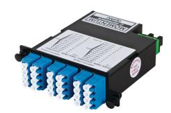
Infinium M4 pre-terminated cassettes with method B provide rapid deployment and have a flipped polarity inside the modules, which use key-up to key-up MPO adapters and allows for straight through patching. The rugged metal housing offers additional durability and includes a built-in internal bend limiting feature to assure optimum optical performance.
