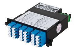
Infinium M4 pre-terminated cassettes with method B provide rapid deployment and have a flipped polarity inside the modules, which use key-up to key-up MPO adapters and allows for straight through patching. The rugged metal housing offers additional durability and includes a built-in internal bend limiting feature to assure optimum optical performance.
