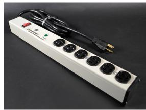
Perma Power computer grade surge protection. Six outlets, lighted switch, durable putty white aluminum housing, 20A. 15' (4.6m) 12/3 SJT putty white cord with NEMA5-15 plug. Length 18"" (457mm). Snap-on, slide-off mounting.
