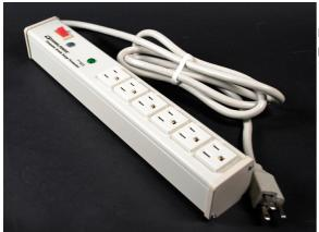
Perma Power computer grade surge protection. Six outlets, lighted switch, durable putty white aluminum housing, 15A. 6' (1.8m) 14/3 SJT putty white cord with NEMA5-15 plug. Length 16"" (407mm). Snap-on, slide-off mounting.
