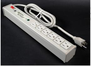
Sentrex high performance surge protection. Six outlets, lighted switch, durable putty white aluminum housing, 15A. 15' (4.6m) 14/3 SJT putty white cord with NEMA5-15 plug. Length 15 1/4"" (387mm). Snap-on, slide-off mounting.
