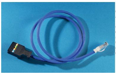
Clarity 110 patch cords are ETL verified to Category 6 and 5e component standards. More importantly, Clarity 110 plugs utilize an internal signal feedback technique to control cross talk without compromising impedance. Clarity 110 to modular 8 position patch cords utilize both signal feedback and center tuning. This allows more transparent connector interfaces for significant elevation of channel performance that can be field measured.
