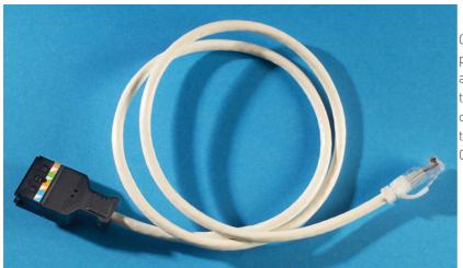
Clarity 6 Patch Cord, Category 6, modular 8position to 110. Cord is terminated on one end with a male 110 plug with internal signal feedback technology, which reduces crosstalk without compromising impedance. The other cord end is terminated with an 8-position modular plug with Ortronics Paralign 2 pair isolation technology.
