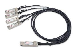
0.5m Mellanox MC2609130-050 Compatible 40GBase-DAC QSFP+ to 4 x SFP+ Breakout (Passive Twinax Copper, PVC) Direct Attach Cable
