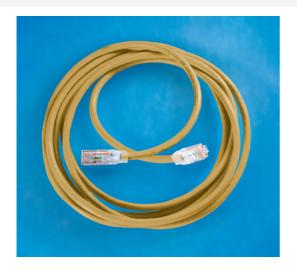
Clarity 5E Premium Category 5e Modular Patch Cord, yellow, 15', Category 5e, four-pair UTP stranded 24 AWG PVC/CM, center tuned with Clarity 5E connecting hardware for optimum Category 5e installed performance using Ortronics Paralign 2 pair-positioning technology
