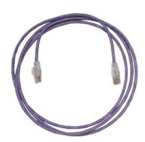
Clarity 5E Premium Category 5e Modular Patch Cord, purple, 15', Category 5e, four-pair UTP stranded 24 AWG PVC/CM, center tuned with Clarity 5E connecting hardware for optimum Category 5e installed performance using Ortronics Paralign 2 pair-positioning technology
