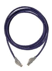
Clarity 6 Modular Patch Cord, purple, 3', Category 6, four-pair UTP stranded 24 AWG PVC/CM, center tuned with Clarity 6 connecting hardware for optimum Category 6 installed performance using Paralign 2 pair-positioning technology
