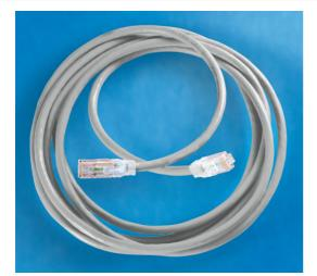
Clarity 6 Modular Patch Cord, white, 3', Category 6, four-pair UTP stranded 24 AWG PVC/CM, center tuned with Clarity 6 connecting hardware for optimum Category 6 installed performance using Paralign 2 pair-positioning technology
