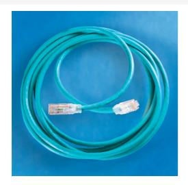
Clarity 6 Modular Patch Cord, blue, 4', Category 6, four-pair UTP stranded 24 AWG PVC/CM, center tuned with Clarity 6 connecting hardware for optimum Category 6 installed performance using Ortronics Paralign 2 pair-positioning technolgy
