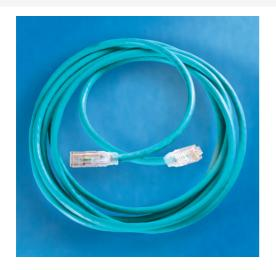
Clarity 6 Modular Patch Cord, blue, 4', Category 6, four-pair UTP stranded 24 AWG PVC/CM, center tuned with Clarity 6 connecting hardware for optimum Category 6 installed performance using Ortronics Paralign 2 pair-positioning technology
