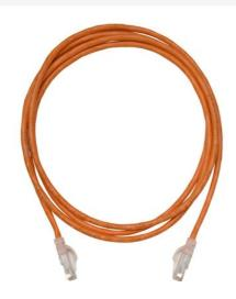
Clarity 6 Modular Patch Cord, orange, 25', Category 6, four-pair UTP stranded 24 AWG PVC/CM, center tuned with Clarity 6 connecting hardware for optimum Category 6 installed performance using Ortronics 'Paralign 2' pair-positioning technology
