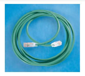
Clarity 6 Modular Patch Cord, green, 25', Category 6, four-pair UTP stranded 24 AWG PVC/CM, center tuned with Clarity 6 connecting hardware for optimum Category 6 installed performance using Ortronics "Paralign 2" pair-positioning technology
