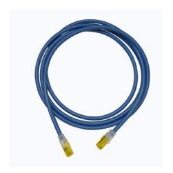
Clarity 6A modular patch cord, blue, 5', Cat6A, 10 Gigabit, four-pair UTP stranded 26 AWG PVC/CM, center tuned with Clarity connecting hardware for optimum installed performance using Ortronics Paralign 2 pair-positioning technology.
