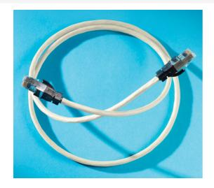
Clarity 6 Shielded, Modular Patch Cord, gray 9', Category 6, four-pair shielded stranded 27 AWG PVC, center tuned with Clarity 6 shielded connecting hardware to provide a significant elevation of channel performance that can be field measured
