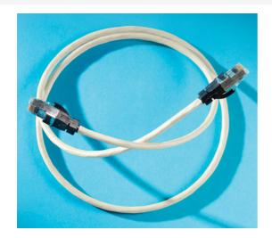
Clarity 6 Shielded, Modular Patch Cord, gray 25', Category 6, four-pair shielded stranded 27 AWG PVC, center tuned with Clarity 6 shielded connecting hardware to provide a significant elevation of channel performance that can be field measured
