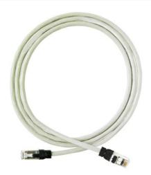
Clarity 6A FTP Modular Patch Cord, red, 5', Category 6A, four-pair FTP stranded 26 AWG PVC/CM, center tuned with Clarity 6 A connecting hardware for optimum Category 6A installed performance using Shielded Paralign 2 pair-positioning technology.
