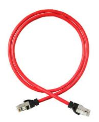
Clarity 6A FTP Modular Patch Cord, red, 7', Category 6A, four-pair FTP stranded 26 AWG PVC/CM, center tuned with Clarity 6 A connecting hardware for optimum Category 6A installed performance using Shielded Paralign 2 pair-positioning technology.
