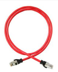
Clarity 6A FTP Modular Patch Cord, red, 9', Category 6A, four-pair FTP stranded 26 AWG PVC/CM, center tuned with Clarity 6 A connecting hardware for optimum Category 6A installed performance using Shielded Paralign 2 pair-positioning technology.
