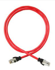
Clarity 6A FTP Modular Patch Cord, red, 9', Category 6A, four-pair FTP stranded 26 AWG PVC/CM, center tuned with Clarity 6 A connecting hardware for optimum Category 6A installed performance using Shielded Paralign 2 pair-positioning technology.
